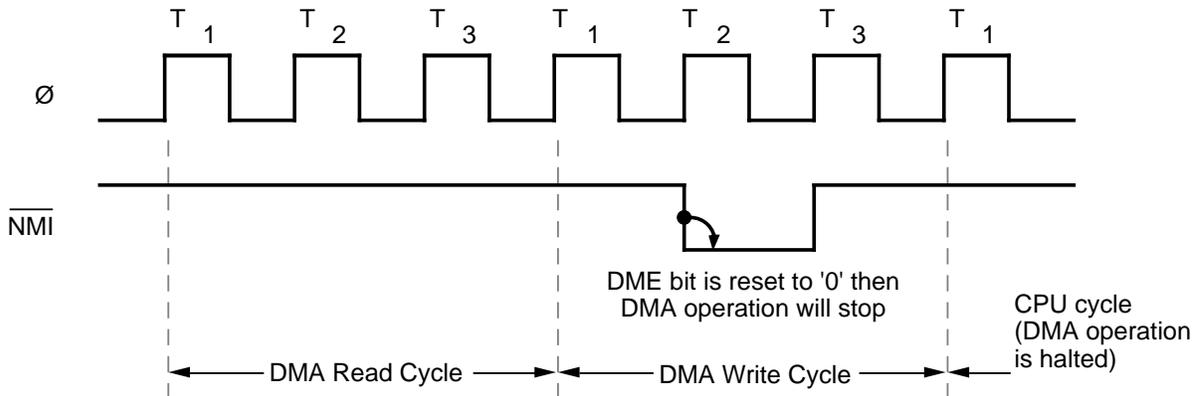
To restart DMA after the /NMI processing, DE (DE0 or DE1) bit should be set to 1 along with DME bit to 1.
