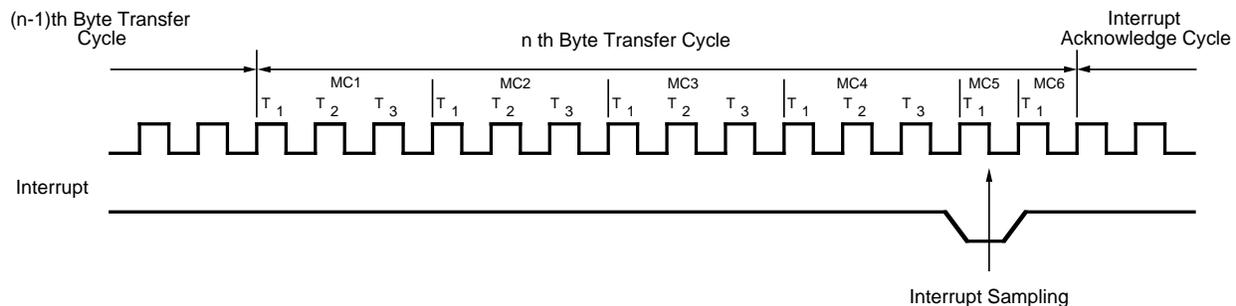
**Q: During interrupt Mode 0, if a call instruction is put onto the bus during the interrupt acknowledge cycle, software won't return the correct address. Why?**
