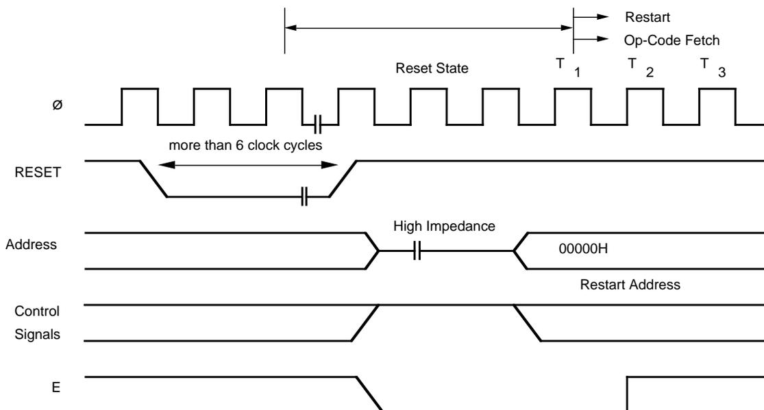
**Note:** /RESET pin should be asserted Low for at least 6 clock cycles to perform power-on reset correctly.
